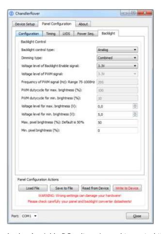
**Backlight control type**: Analog (variable DC voltage is used to control the brightness) or PWM (brightness is controlled by the duty cycle of a PWM signal).
