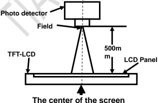
Note 2: Definition of viewing angle range and measurement system. viewing angle is measured at the center point of the LCD.
