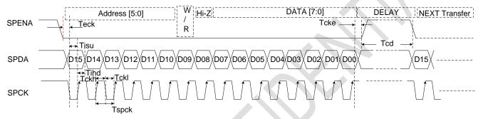
Note: DDLY Description (Ths= DDLY+ Offset) R04: Source Timing Delay Control Register
