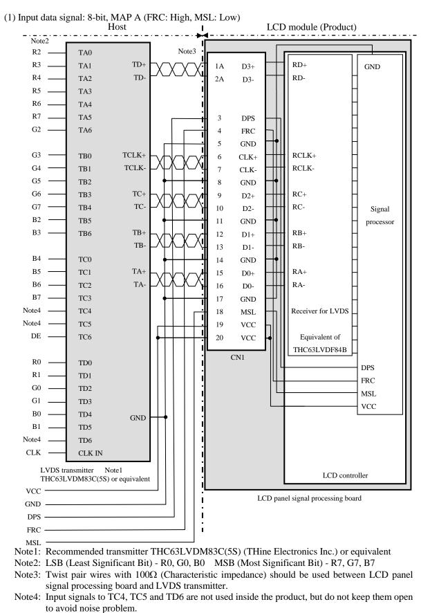
4.5.4 Connection between receiver and transmitter for LVDS
