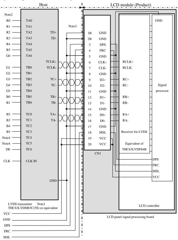
(3) Input data signal: 6-bit (FRC: Low or Open, MSL: Low)
