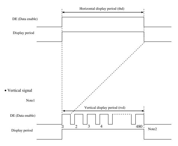
Note1: This diagram indicates virtual signal for set up to timing. Note2: See "**4.9.3 Input signal timing chart**" for the pulse number.
