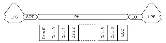
LPS: Low power state SOT: Start of Transmission PH: Packet Header
