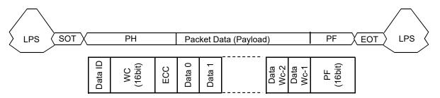
LPS : Low power state SOT : Start of Transmission PH : Packet Header
