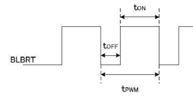
Please do not set  $t_{OFF}$  with  $0 \ \mu s < t_{OFF} < 1 \ \mu s$ . In case of lower frequency, the deterioration of the display quality, flicker etc., may occur.
