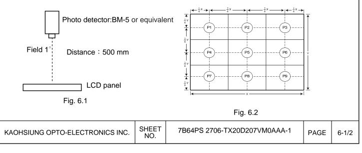
Note 3: The Contrast ratio is measured from the center point of the panel, P5, and defined as the following equation:
