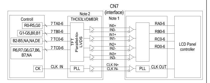
Note 1: LVDS cable impedance should be 100 ohms per signal line when each 2-lines (+, -) is used in differential mode.
