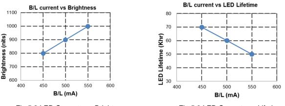
Fig 5.2 LED Current v.s. Brightness
