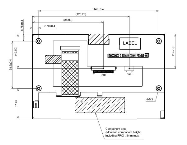
General Tolerance:±0.5mm Scale : NTS Unit : mm
