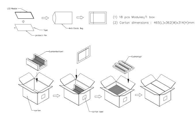
Figure. 9-1 Packing method
