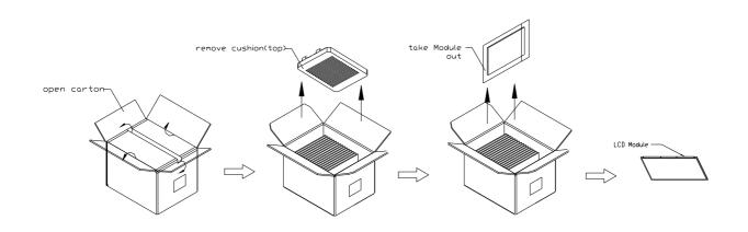
Figure. 9-3 UN-Packing method
