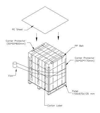
Figure. 9-2 Packing method
