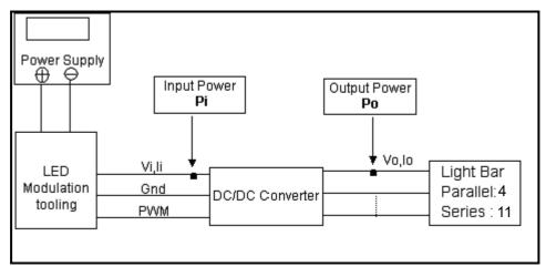
Note (2) At 190 ~1kHz PWM control frequency, duty ratio range is restricted from 5% to 100%.
