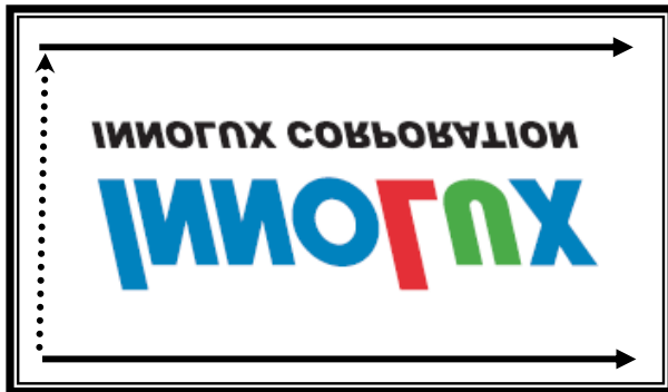
Fig. 1 Normal scan ( pin 17, LR = High ; pin 18, UD = Low )
