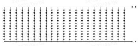
Figure 3-1 Front Light Circuit
