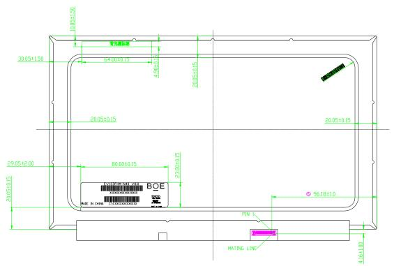
Figure 22. TFT-LCD Module Outline Dimensions (Rear view)
