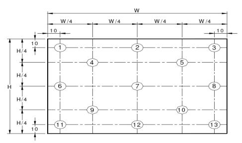
Figure 9. Uniformity Measurement Locations (13 points)
