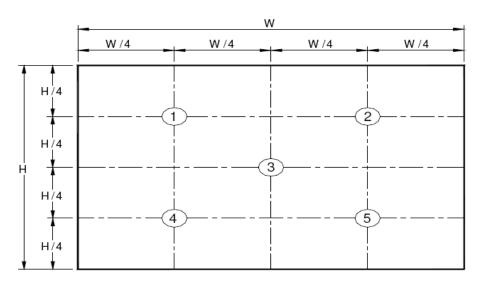
Figure 8. White Luminance and Uniformity Measurement Locations (5 points)
