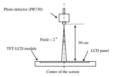
Optical characteristics measurement setup
