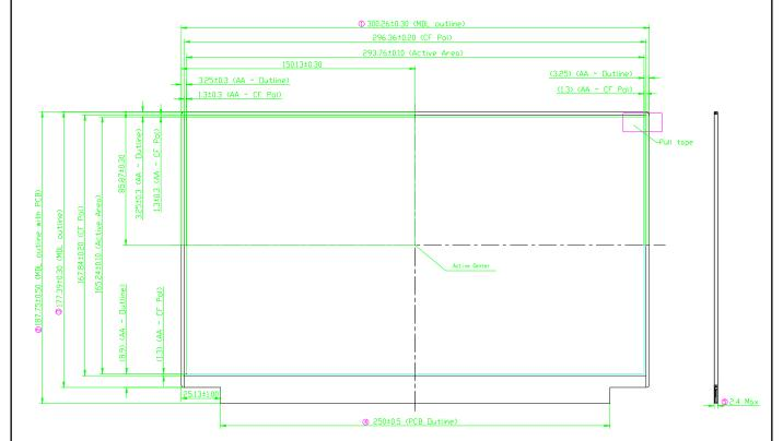
Figure 20. TFT-LCD Module Outline Dimension (Front View)
