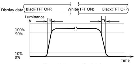
Figure 10. Response Time Testing
