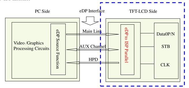
Figure 12. eDP Interface Architecture
