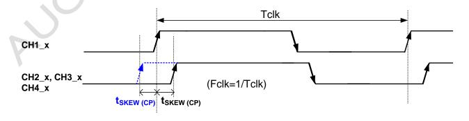
Note3. LVDS Receiver Clock SSCG (Spread spectrum clock generator) is defined as below figures.
