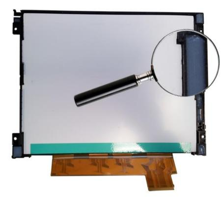
We complete all small recesses and the honeycomb structure of the bezel with silicone
