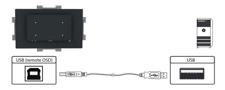
Connecting the touch to a PC with USB cable (for displays with touch sensor only)
