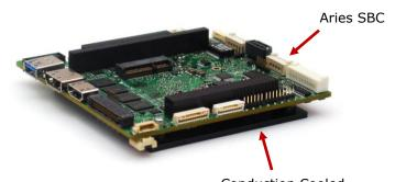
Conduction Cooled Heat Spreader
