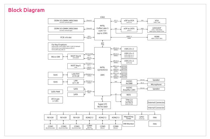
1 x LVDS internal connector, dual channel, resolution up to 1920 x 1200 @ 60Hz (eDP: by request)
