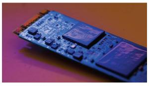
A Transcend M.2 SSD with acrylic conformal coating under UV light inspection
