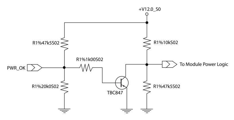
The voltage divider ensures that the input complies with 3.3 V CMOS characteristic and also makes it possible to use the module on carrier board designs that do not drive the PWR\_OK signal. Although the PWR\_OK input is not mandatory for the onboard power-up sequencing, it is strongly recommended that the carrier board hardware drives the signal low until it is safe to let the module boot-up.
