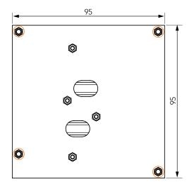
M2.5 x 11 mm threaded standoff for threaded version or ø2.7 x 11 mm non-threaded standoff for borehole version
