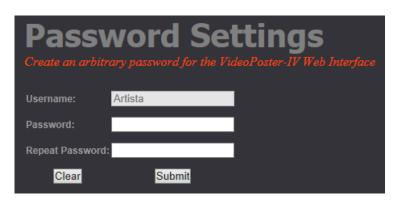
The new password must be entered twice to prevent the device from being inaccessible due to typing errors. Form data can be reset by clicking "Clear". By pressing "Submit" the new password will be activated and you will have to re-login on changing to any other page of the web frontend.
